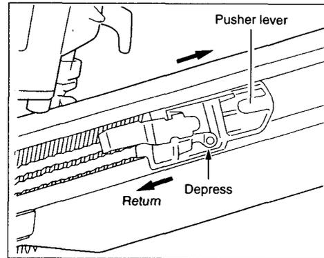
Depress the nail stopper and remove the strip of nails from the magazine.
